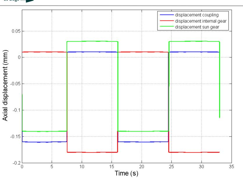
Axial displacements of gear wheels
