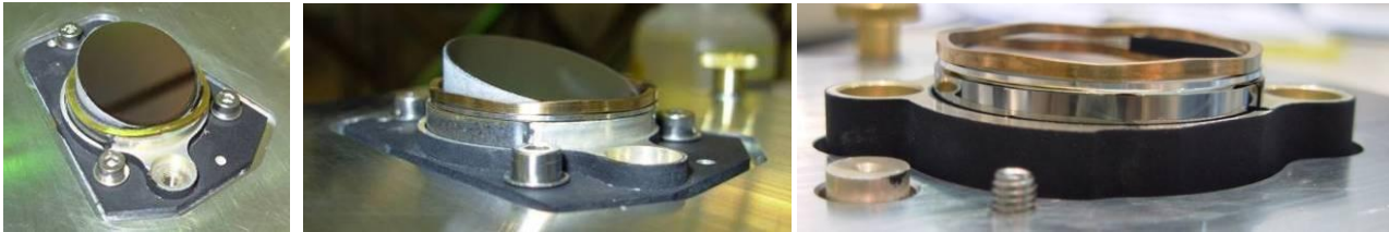
Fig. 2: Flight Model Integration of the DPA; view of the first gold washer (left); the stack of four ZnS washers (middle); the stack of four Ge washers (right); covers of the prisms not integrated
