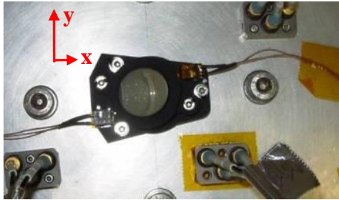
Fig. 16: Qualification Vibrations: Pilot Accelerometers Levels
