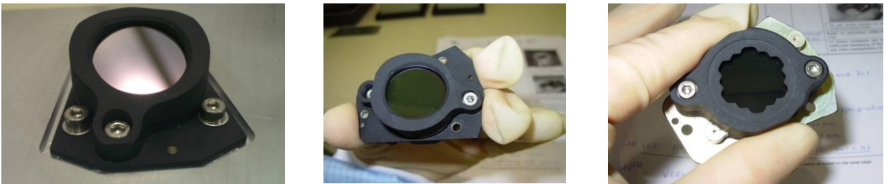
Fig. 3: Flight Model of the DPA; views onto the ZnS side (left/middle) and onto the Ge side (right); covers are integrated and maintain the prisms on the holder
