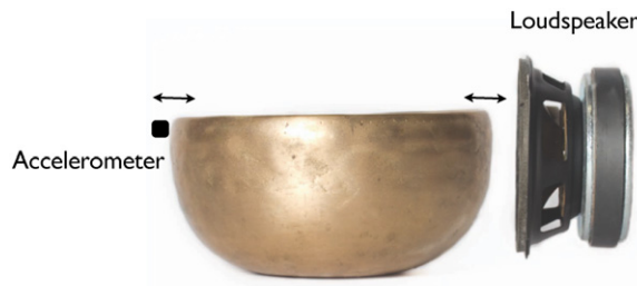
Figure 6. Experimental setup. The bowl deformation is excited by a loudspeaker emitting sound at a frequency corresponding to a particular vibrational mode of the bowl. The deformation of the bowl is measured by an accelerometer glued to the bowl's outer wall at the height of the liquid surface.
