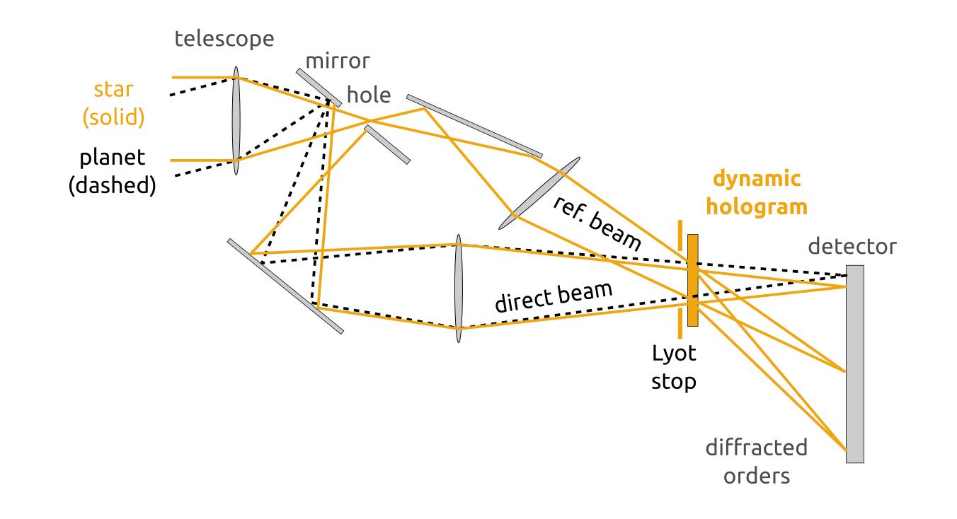
The two beams create fringes in the speckles of the hologram → recording the hologram.
