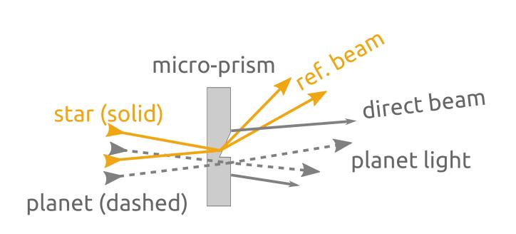
More performing design: the hole in the flat mirror is replaced by a micro-prism. This approach is presented in our recent papers:
