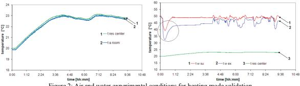
Figure 2: Air and water experimental conditions for heating mode validation
