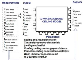
Figure 1: Definition of the cooling ceiling model inputs outputs and parameters
