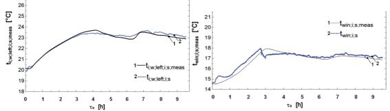
Figure 3: Comparison: Measured and calculated temperatures of internal wall and window at the internal surface.
