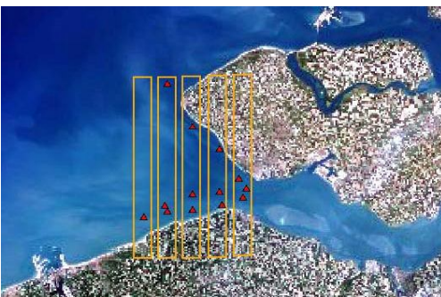
Figure 1: Scheldt test site: CASI five flight lines, the triangles represent the location of 12 in situ survey stations.
