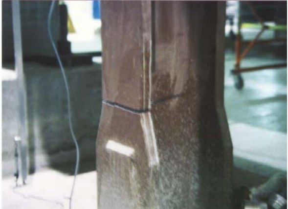
Picture 3.3.3. Fracture of the dog bone after phase 5.
