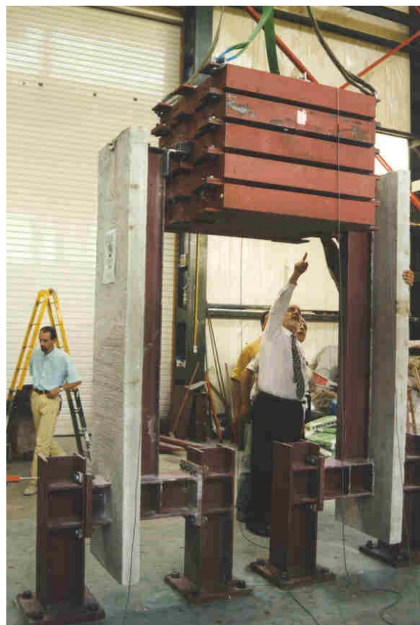
Figure 3.11.4 Experimental set-up and instrumentation in shaking table tests
