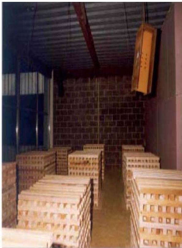
Fire load by 45 standard wooden cribs
