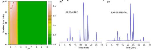
Figure (a) depicts the probability surface to obtain a separation (*S*) of at least 0 min (baseline resolved peaks). The quality level is set to 85% and the corresponding design space is surrounded in red. Figure (b) displays the predicted chromatogram at pH 3.0 and with a gradient time of 30 min. (within the DS). Figure (c) shows the chromatogram recorded at this operating condition.
