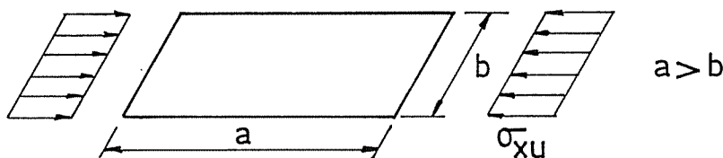
Figure IV.28 : Compression uniforme axiale
