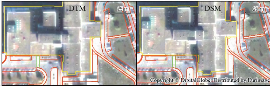
Figure 5. The hospital corners fit better the vector with orthorectification done with DSM (right).
