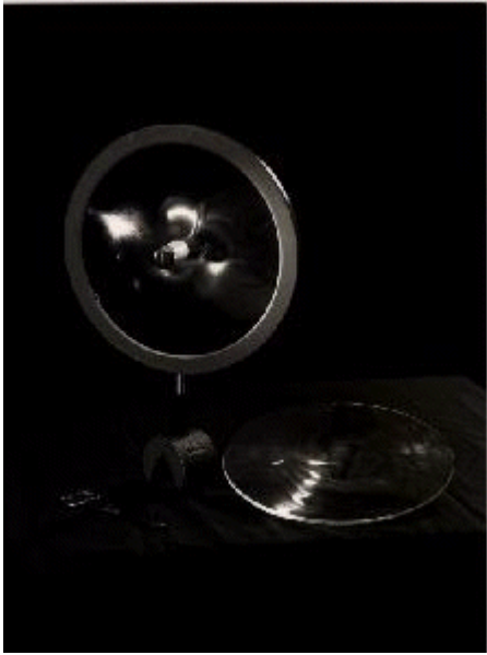
Figure 3: Examples of a 'point mass' (left) and a 'spiral galaxy' (right) optical lens produced by the authors. We have used these particular lenses, made of plexiglas-like material ( n = 1.49 , 30 cm in diameter), to simulate the formation of multiple images of a distant source. The optical gravitational lens experiment is described in section 4.
