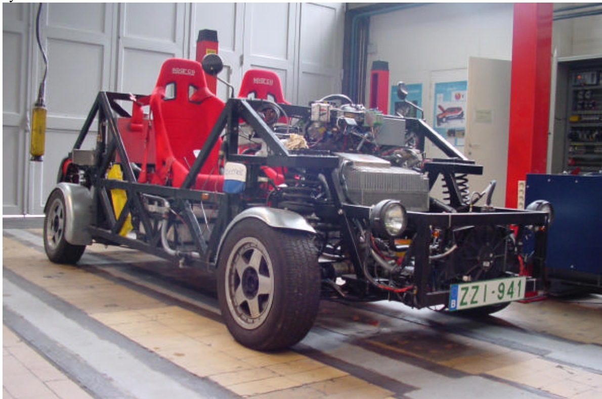
Fig. 13 the ULg parallel hybrid car used for the test on roller bench. The Ni-Cd batteries are located below the seats.(courtesy : Mécanique du Transport, Université de Liège). The SCADA is using two data logger Fluke NetDAQ 2645 A (20 inputs), piloted by PC.
