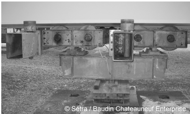
Figure 7-3: Launching shoe with 4 wheels and 2 lateral wheels for longitudinal guidance (total length = 1.25 m).
