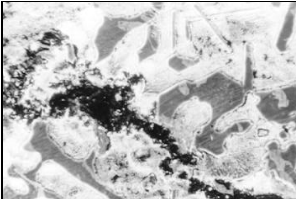
Fig.9 - Microstructure of heat treated sample - (resistivity - 1100°C - 5°/min) SEM - etched sample.
