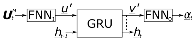
Figure 2. Schematic of the RNN. The three components of \mathbf{U}_t^M (at time increment t ) are the input variables and the n_m coefficients of \alpha_t (at time increment t ) are the output variables. FNN I and FNN O are each a single layer feed-forward neural network. The GRU's input is the output of FNN I (denoted by \underline{u}' ), as well as the hidden states the GRU has predicted for the previous time increment, \underline{h}_{t-1} (i.e. at time t - 1 ). The GRU's primary output, \underline{v}' , serves as the input for FNN O , as well as updated hidden states, \underline{h}_t , that the GRU will use as input for the next time increment, i.e. at t + 1 .
