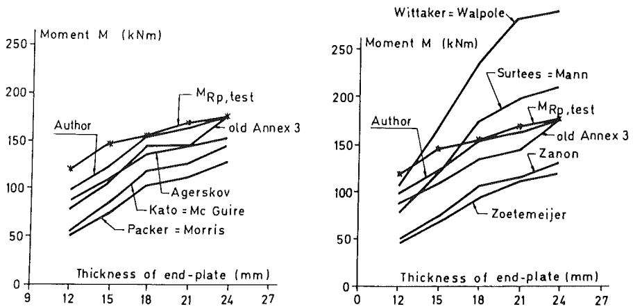
Figure 11 Test-model comparisons for isolated end-plates (T-stub models).
