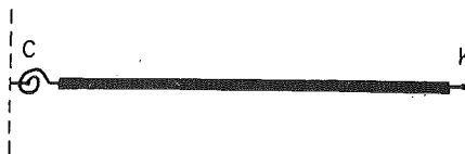
(b) Simplified "beam + joint" modelling (recommended in Eurocode 3)
