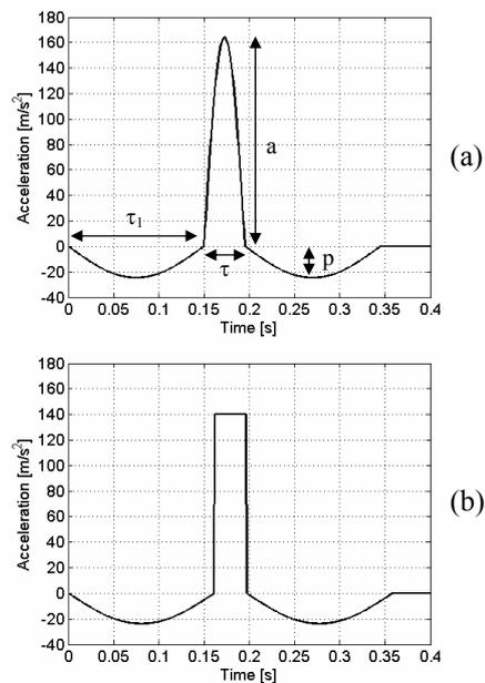
Fig. 7. Examples of shock specification ( $a$  = peak pulse,  $\tau$  = pulse length,  $p$  = pre/post pulse amplitude,  $\tau_1$  = pre/post pulse length) : (a) Half-sine/single sided pulse; (b) Rectangular pulse
