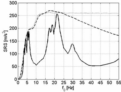
**Fig. 8.** Comparison between the *SRS* of shock specifications and of the vibration environment of the *NEMO* lighting device for  $\epsilon = 5\%$  (---, Half-sine/single sided pulse; ···, Rectangular pulse; —, Envelope of the computed *SRS*)
