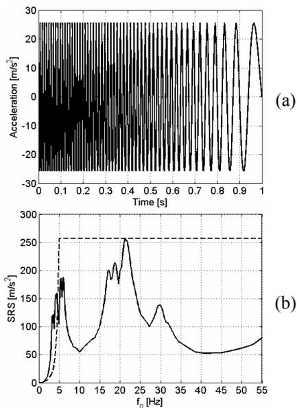
**Fig. 9.** Example of sine sweep excitation: (a) Control time sample; (b) *ERS* and *SRS* for  $\epsilon = 5\%$  (---, Sine sweep excitation; —, Envelope of the computed *SRS*)
