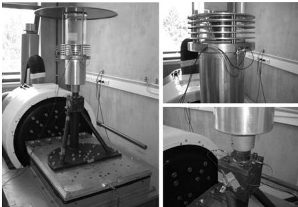
**Fig. 11.** View of the *NEMO* lighting device ready to be tested on the *Gearing & Watson* 26 kN electrodynamic shaker
