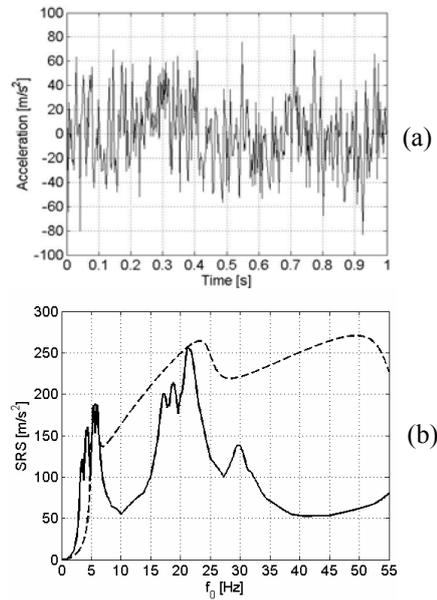
**Fig. 10.** Example of random excitation: (a) Control time sample; (b) *ERS* and *SRS* for  $\epsilon = 5\%$  (---, Random excitation; —, Envelope of the computed *SRS*)
