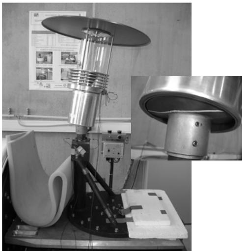
**Fig. 16.** View of the failure induced to the NEMO lighting device at the end of the “impact test”
