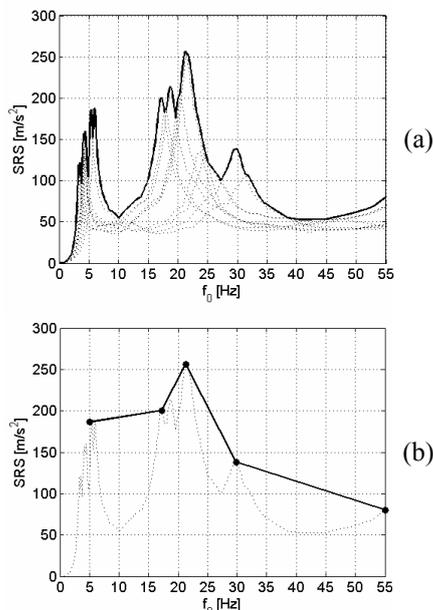
Fig. 5. Testing specification equivalent to an impact on the pole : (a) Envelope of the *SRS* computed from the responses of the different poles at the fixing point of the lighting device for  $\varepsilon = 5\%$ ; (b) Envelope to be used for vibration testing on electrodynamic shaker
