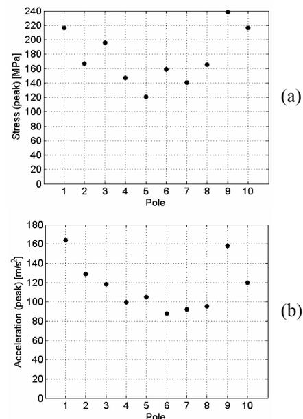
**Fig. 3.** Peak responses computed for the whole set of *NEMO* poles ( $\varepsilon = 0.05$  %) : (a) Stress at the base of the pole (point 1); (b) Acceleration at the fixing point of the lighting device on the pole (point 2) in the  $ox$  direction
