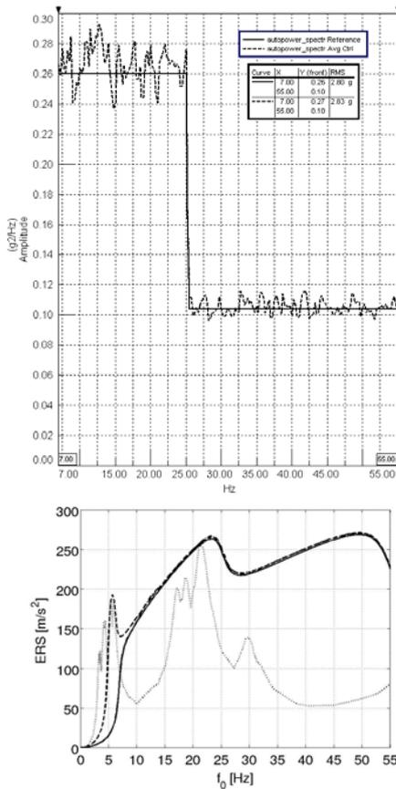
**Fig. 15.** Random specifications and ERS for  $\epsilon = 5\%$  (- - -, Initial specification; —, Modified specification; · · ·, Control specification; · · ·, Envelope of the computed SRS)
