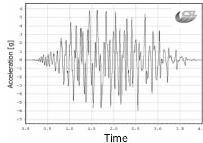
Fig. 6. Example of time sample corresponding to the *SRS* of Fig. 6 (b) (generated with the *VibExec* vibration control system, *m+p international*, provided by *CSL – University of Liège*)
