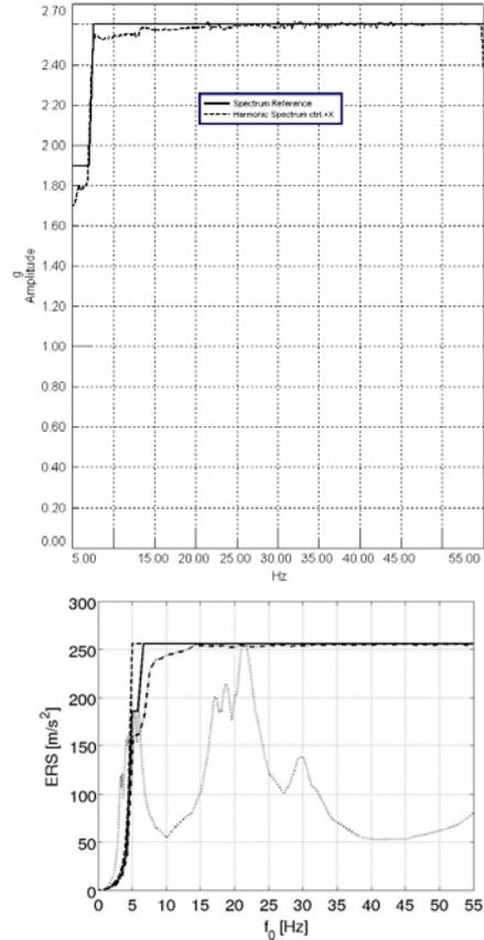
**Fig. 14.** Sine sweep specifications and ERS for  $\epsilon = 5\%$  ( - - -, Initial specification; —, Modified specification; · · ·, Control specification; · · ·, Envelope of the computed SRS)
