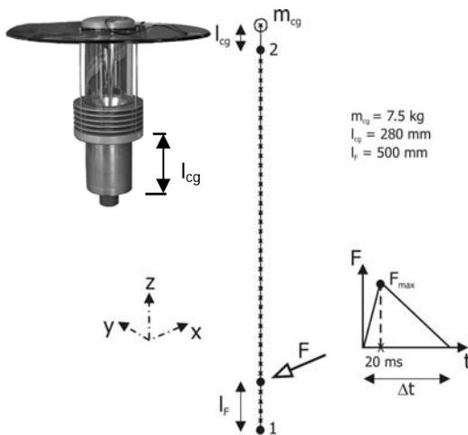
**Fig. 1.** Finite element model of the NEMO "pole/lighting device" system subject to an impact
