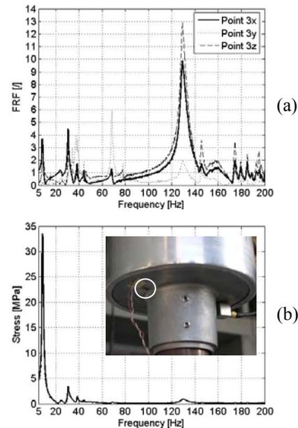
**Fig. 12.** Low level sine sweep : (a) *FRF* between the responses of the main body (point 3) and the excitation at the fixing point; (b) Stress measured on the external face of the fixing part
