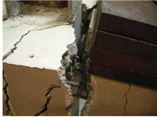
Figure III.45. Collapse of the longitudinal rebars in the vicinity of the external composite joints at point “D” of Figure III.39
