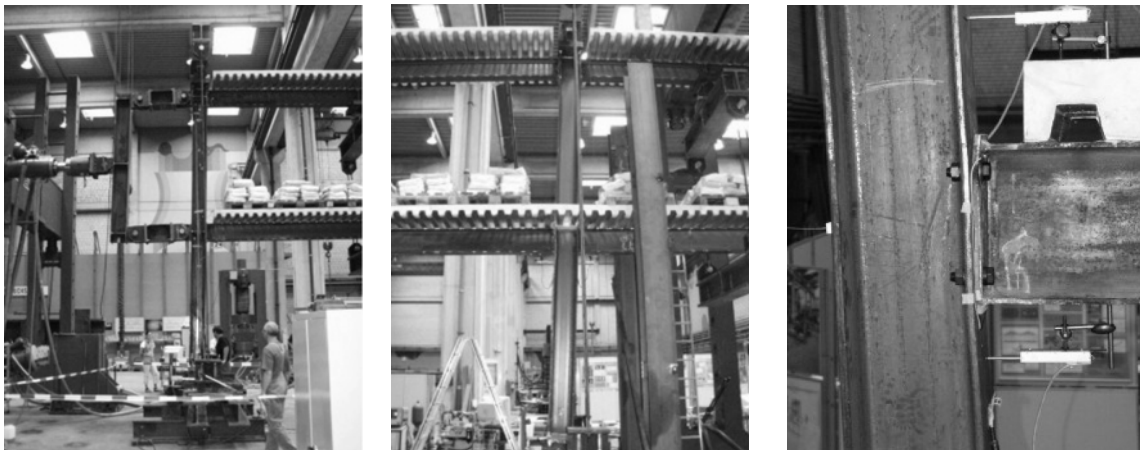
Figure II.59. Deformation of the “Bochum” frame at the end of the test [1]
