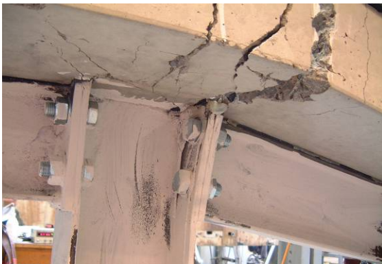
Figure III.46. Yielding spread in the steel components of the external composite joints
