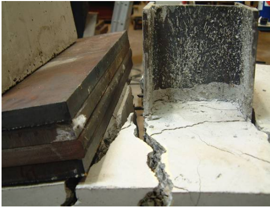
Figure III.45. Collapse of the longitudinal rebars in the vicinity of the external composite joints at point “D” of Figure III.39
