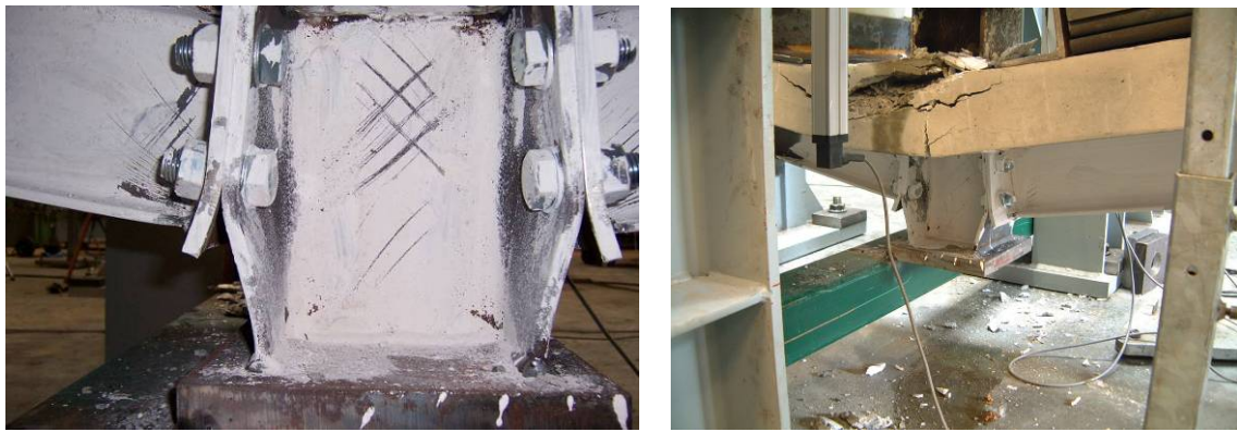
Figure III.53. Internal composite joints at the end of the test
