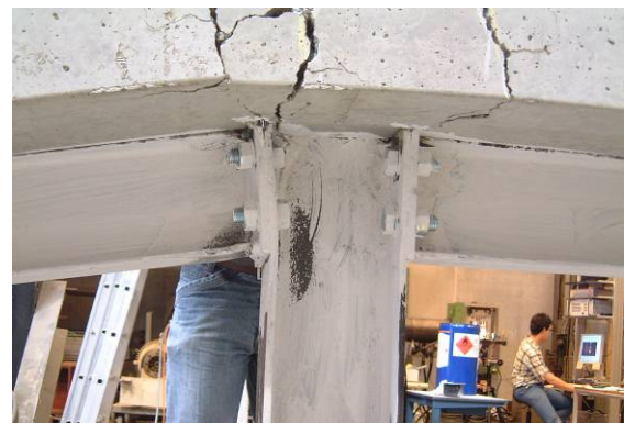
Figure III.46. Yielding spread in the steel components of the external composite joints
