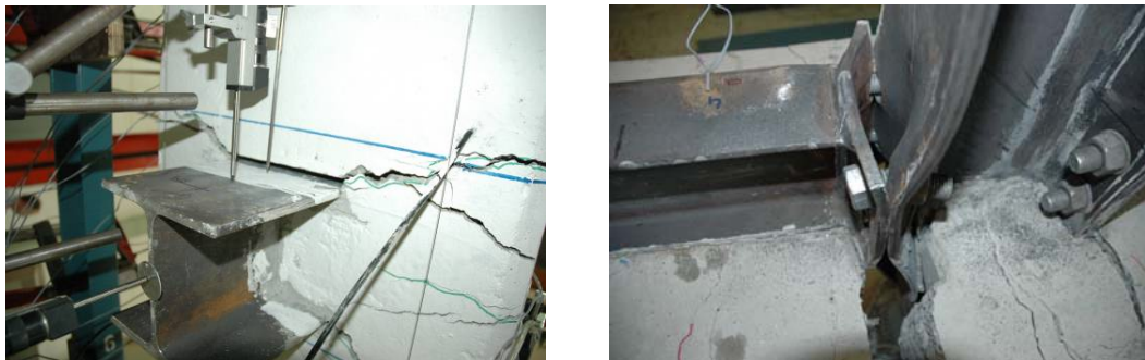
Figure III.63. Tested specimen subjected to hogging bending moments and tension loads at the end of the test
