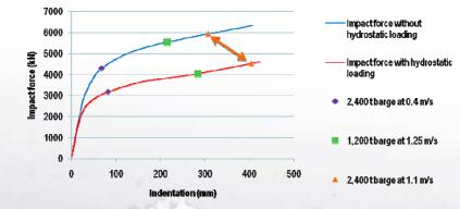
The global behaviour of the gate is identical but the structure is more deformable because previously submitted to a stress field
