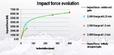
By using class-1 sections for frames and girders, we improve the gate behaviour in case of ship impact
