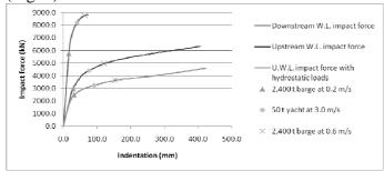
Figure 2. Impact force evolution for different impact cases.
