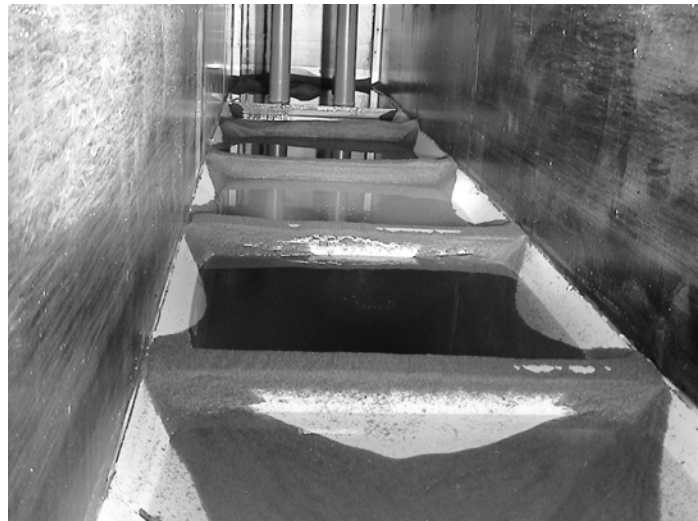
Fig. 6 View of the interior of a chamber after a sedimentation test
