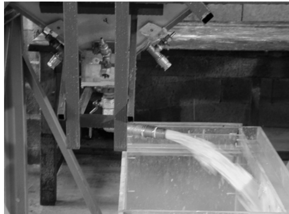
Fig. 4 Hopper flushing operation
