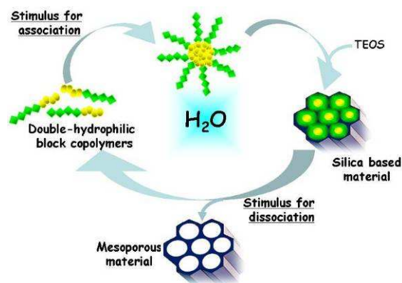
Figure 1: General strategy for structuring silica using induced and reversible micelles of water-soluble block copolymers. Porosity is created at room temperature, while the structuring agent is recycled in aqueous solution. TEOS=tetraethoxysilane.
