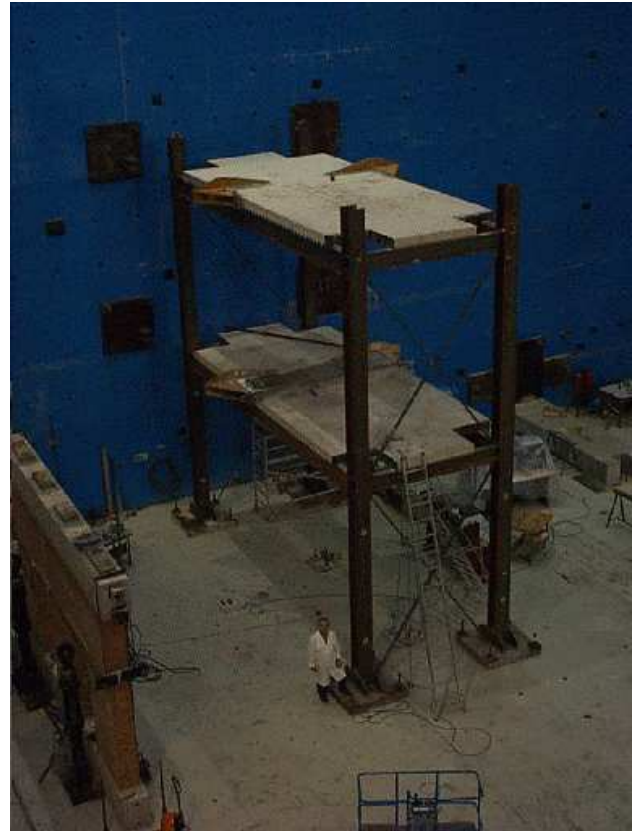
Figure 1: The STEELQUAKE structure.
