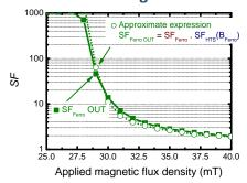
In the Ferro OUT configuration, the SF of the hybrid tube is approximately given by the product of the SF of the single tubes
