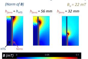
Reduction of the shielded domain if  $h_{Ferro}$  is reduced
