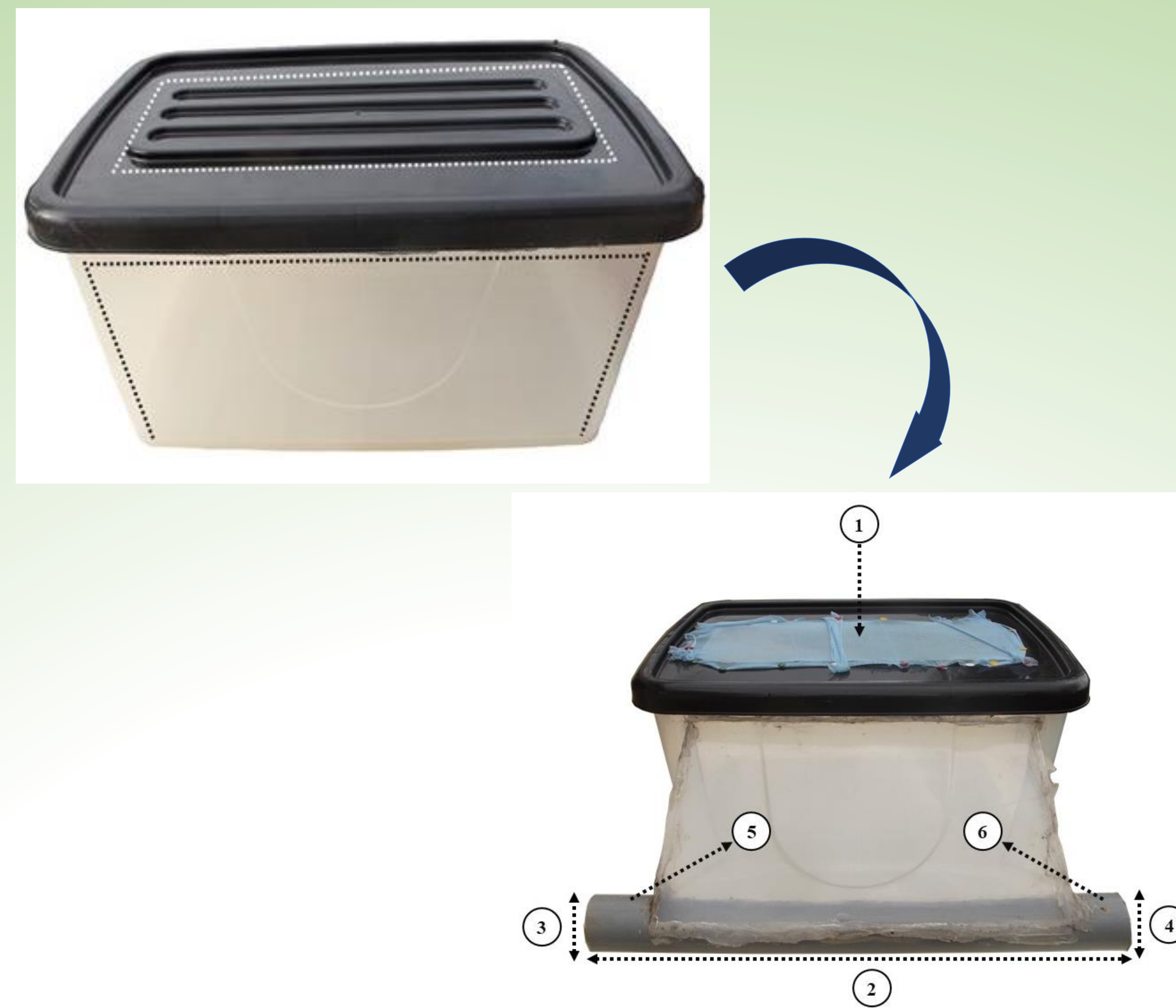
Figure 1: Prototype of larvarium. The dots represent the cut lines. 1: window opening covered by a mosquito net, 2: prepupae collection trough, 3: exit for the prepupae, 4: closed end, 5 and 6: prepupae exit ramp.
