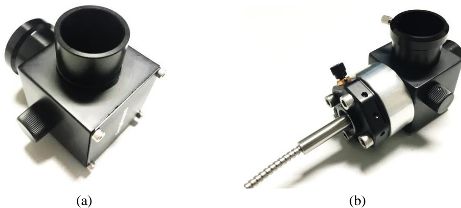
Figure 13. Flipping mirror device: the upper flange connects to the telescope, the left connecting tube intends to hold an eyepiece and the lower hidden aperture incorporates a standard thread for cameras. The small turning button activates the flipping mechanism (a). Fiber bundle connected to flipping device with translation mount and custom flange.
