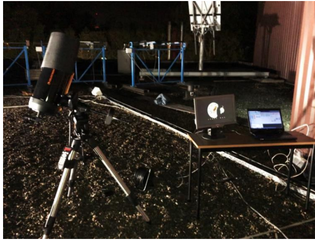
Figure 12. Observation setup installed on CSL facilities roof. The laptop was dedicated to the spectrograph control.
