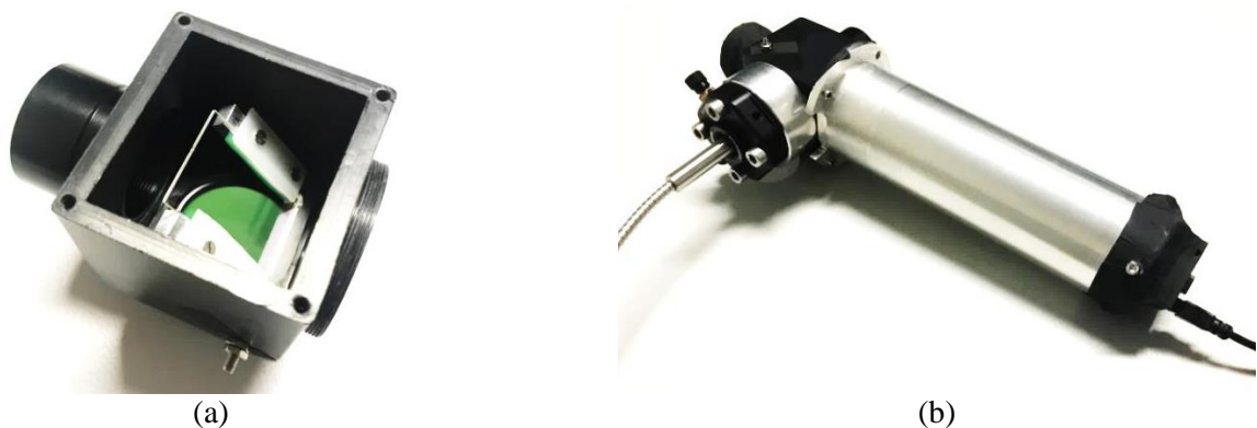
Figure 15. Modified flipping mirror box (a) and adapted tracking device (b).
