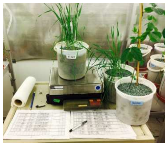
Figure 1. Daily gravimetric analysis. The pot surface is covered with blue plastic beads to minimize soil evaporation
