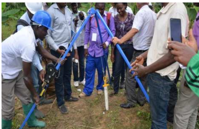
Extracting an access tube that was improperly installed. (Photo: IRAD)
