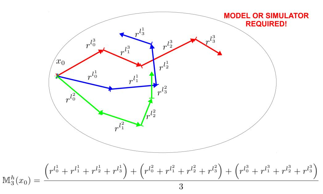
If the system dynamics and the reward function were accessible to simulation, then **Monte Carlo (MC) estimation** would allow estimating the performance of *h*
