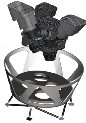
Figure 4. Left. —Diagram illustrating the orientations of the four TESS cameras, lens hoods, and mounting platform. Right. —Artist's conception of the TESS spacecraft and payload.
