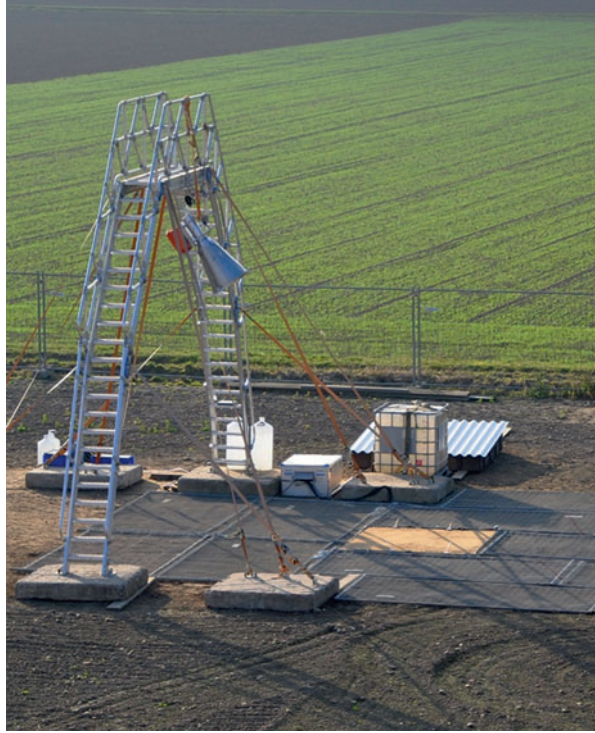
Fig. 3 Controlled setup for active and passive microwave remote sensing studies at the TERENO test site in Selhausen, Germany. The setup consists of an ELBARA II radiometer mounted on an arc and a sand box in the center of a wire grid.
