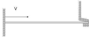
Figure 13: Model of dynamic buckling of a cylinder
