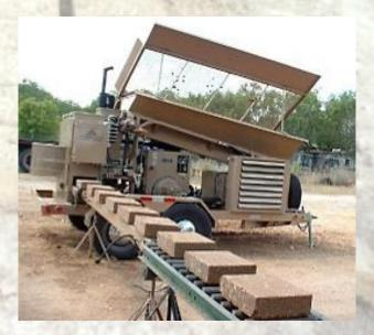
Compressed Earth Brick (CEB): compacted earth, achieved using manual or mechanical presses.
