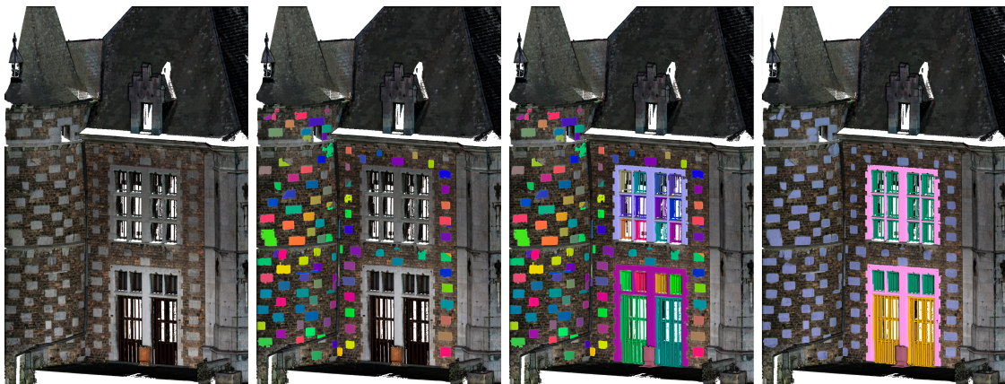
Figure 12. Ontology-based classification of the South-South-West façade of the castle of Jehay. From left to right: the façade studied; the result of the segmentation (stones only); the result of the full segmentation; the result of the classification for quasi-planar objects of interest.
