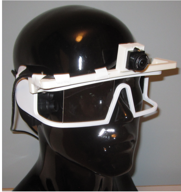
FIGURE 3.3: The second prototype we used for the head-mounted device, adapted from a Drowsimeter R100 provided by Phasya S.A. (Angleur, Belgium).
