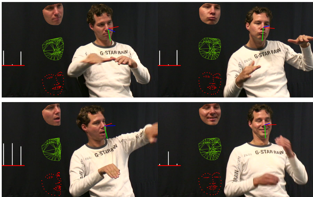
FIGURE 2.8: Extraction of sign language facial cues from a video of a signer from the NGT corpus [72]. The axis system attached to the signer's face gives a visual impression of the rotation around, and translation along, the X-axis (red bar), Y-axis (green bar), and Z-axis (blue bar). The three white vertical bars in the left part of the images represent, from left to right, the left eye opening degree, the mouth opening degree, and the right eye opening degree. In the central region of each image are shown, from top to bottom, the face texture generated with our AAM-based face alignment method, and the face shape obtained with this same method, triangulated (in green), and non-triangulated (red points).
