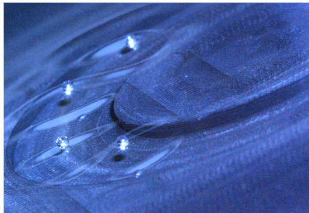
FIGURE 5.9: Four bouncing droplets walking in an annular cavity and creating a coherent wave propelling the group at a speed larger than individual droplets. The coherent wave is seen to follow the cavity symmetry. One can observe anti-synchronous bounces for the successive drops.
