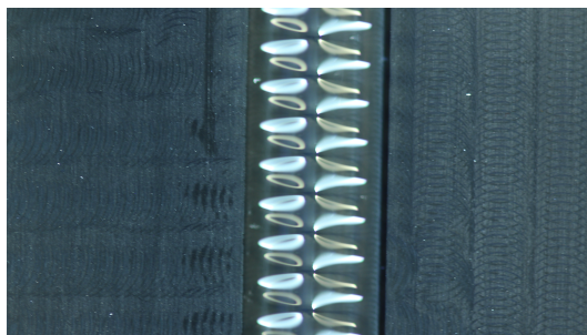
FIGURE 3.14: Faraday instability within a 1.5 \lambda_F channel. One can guess the nodal line at the middle of the channel that splits an antinode of large amplitude from another antinode of lower amplitude.
