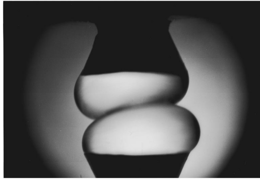
FIGURE 2.3: Photograph of two millimetric droplets. The pendant (sessile) droplet temperature is about 45^{\circ}\text{C} ( 20^{\circ}\text{C} ). When brought in contact no coalescence happens, one can only observe the slipping of both droplets (from [60]).
