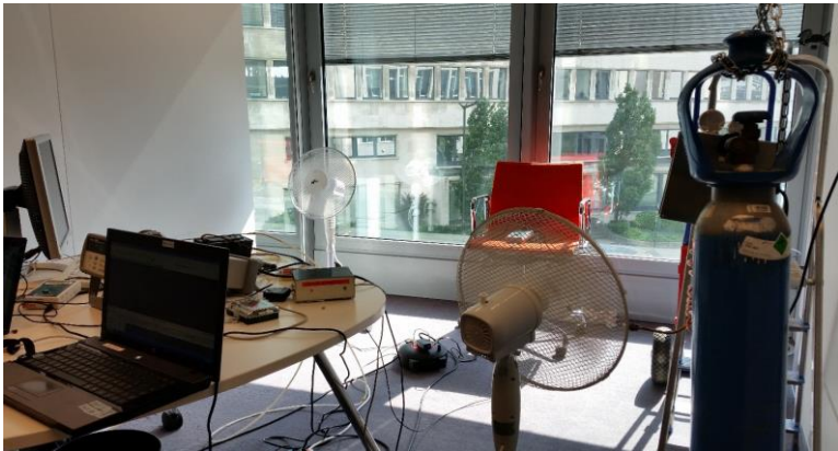
Figure 5 : Tracer gas equipment
