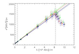
Figure 3.18: Photon transfer curve in linear scale computed for the eight last lines to be read. This procedure emphasizes better the PNCCD saturation depending on the first amplifier range. The saturation happens at ~8000ADU per channel or ~40000e<sup>-</sup> per channel. The dashed-dot vertical lines indicate the photon-noise dominated regime from one  $\sigma_{eRON}$  to saturation.
