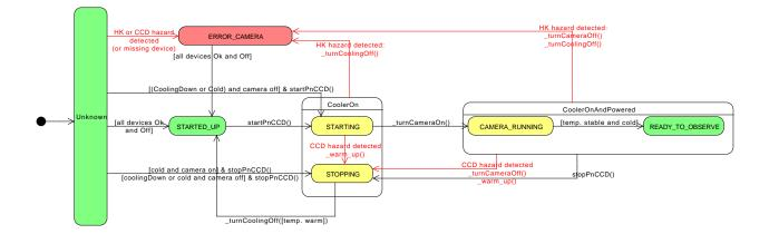
Figure 3.15: PNCCD state machine diagram displaying the possible transitions from states upon "event" being generated by a user (*i.e.* start/stop) or internal (e.g. ready to turn the camera on, hazard detected, etc.). The aim of this state machine is to ensure easy and safe operation. See text for more details.
