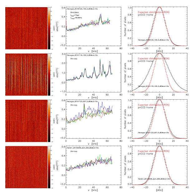
Figure 3.27: *con't*. Based on dark frames offset map corrected and with common-mode correction using the eight covered channels individually for each CAMEX. From top to bottom, the different milestones measurements are : 1) FDR, 2) the 1st version of the LBT Engineer camera - note the difference of scale for the power spectra -, 3) using a manual PSU tower, considered as our "best"/smallest common-mode, 4) the ARGOS final common-mode characterization for the camera LBT#1.
