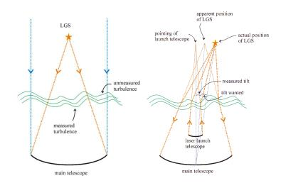
Figure 1.8: (Left) Illustration of the cone effect for a guide star at a finite height. This is also referred as "focus anisoplanatism". (Right) Illustration of the LGS lack of sensitivity to tip-tilt due to the round trip of the laser beam through the atmosphere. Credit : both illustrations are from Davies et al. (2005a),
