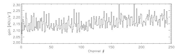
Figure 3.21: Mean gain from channel to channel for one half of the PNCCD. This is obtained with 1000 light and dark frames. Each CAMEX amplifiers behaves slightly differently, whence the small gain variations. The RMS gain variation is < 2% and the PtV is  $\sim 10\%$ .
