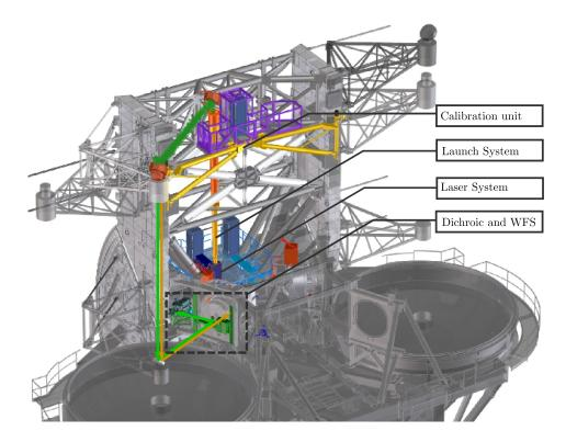
Figure 2.3: CAD model of LBT with the ARGOS hardware (complete for one side). As it can be seen the system is very distributed and the final integration can only be done at LBT. This figure can be read in parallel to Fig. 2.2. The main sub-systems are annotated. The dashed grey box is also represented in Fig. 2.4. The light rays are indicated by arrows from the ASM down to the WFS (green) and to LUCI (orange). Credit: modified from image of M. Deysenroth and H. Gemperlein.
