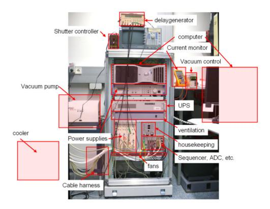
Figure 3.8: Initial PNCCD rack illustrating the bulky and very distributed devices needed to operated the PNCCD, four to five times larger than the final system represented in Fig. 3.9.
