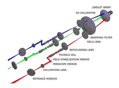
Figure 2.5: Arrangement of the three laser guide stars inside the WFS. Each optical element is annotated and the light paths of the three beams is shown in different colors. The light enters from the right and falls onto the detector on the extreme right. Credit: M. Bonaglia.
