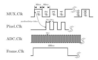
Figure 3.10: "Hand-shake" between CAMEX and ADC clocks. The MUX clock designates the multiplexing clock of the analog pixels at the output of the CAMEX. The other 3 clocks are ADC clocking, with the frame clock marking the start of frame, the ADC clock triggering the ADC acquisition, and the pixel clock selecting the appropriate ADC sample. The delay between the MUX clock and the start of pixel clock has an important effect on the noise quality.
