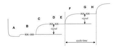
Figure 3.6: "High-speed" timing for the MCDS-filter. (A) is the initial reset of the amplifier and (B) the first baseline. Following this scheme, the amplifier is only reseted at the end of a frame and not after each "cycle time". See also text for more details. Credit: FDR ARGOS consortium (2010), Hartmann et al. (e.g. 2008).
