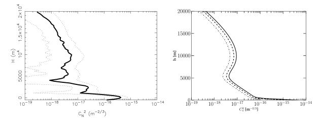
Figure 1.2: (Left) Median  $C_n^2$  profile at Mt. Graham (at the LBT) based on data of 43 nights. The dotted lines indicate the standard deviation. Credit: Masciadri et al. (2010). (Right) Three general atmospheric models based on modified Hufnagel-Valley models. We distinguish three different regimes and use them to compute  $r_0$ ,  $\theta_0$  and  $f_G$ . See Fig. 1.3.
