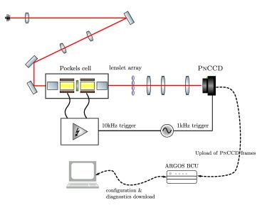
Figure 4.10: Demonstration test bench setup. The red curve is the optical path. Solid black curve are electric signal. Dashed black curves are data signal. See text for a full description.
