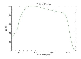
Figure 3.16: Quantum efficiency as optimized for ARGOS obtained by adjustment of antireflective coating. Credit: PNSENSOR.
