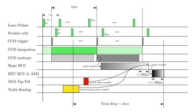
Figure 2.8: ARGOS AO closed-loop timing diagram. It illustrates the nominal timing from laser firing down to deformable mirror control as foreseen by design and estimated in CHAP.3 and in CHAP.4. The total delay between the wavefront measurement and its correction is estimated to < 2ms. The NGS tip-tilt an the "truth sensing" are asynchronous.
