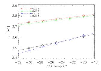
Figure 3.24: Noise versus CCD temperature. Each temperature measurement is done on 1000 frames, median dark subtracted, and full line common-mode corrected. Hence the noise here is the readout noise without the common-mode contribution. A fit by  $\sqrt{aT+b}$  allows us to predict its evolution with temperature. ARGOS will typically operate the PNCCD at  $-25^{\circ}$ C.
