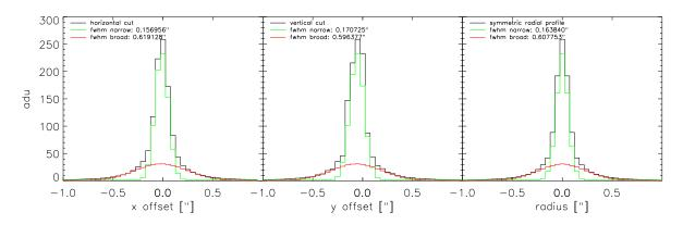
Figure D.3: Horizontal, vertical and symmetric profiles cut of the point spread function as derived from fitting spatially the  $Br\gamma$  line, on the initial data cube (no binning and masking).
