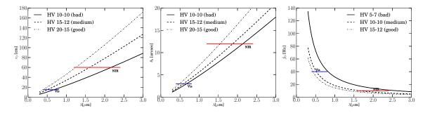
Figure 1.3: Typical parameters computed by using our  $C_n^2$  model in function of wavelength. From left to right : the Fried parameter  $r_0$ , the anisoplanatic angle  $\theta_0$ , and the Greenwood frequency  $f_G$ . In blue and red, the typical visible and near-IR wavelength ranges.
