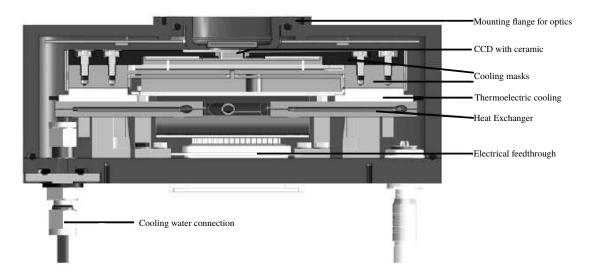
Figure 3.13: Cross-section of the final camera model. The main elements are annotated Light come from top through the entrance window and a few mm below the PNCCD chip. The backplane electronics are here not represented. Credit: Ordavo et al. (2011).
