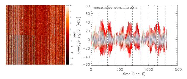
Figure 3.25: Illustration of the common-mode noise at the time of ARGOS FDR. (Left) PNCCD dark frame (N.B. the left halve of the CCD is read to the left, and vice versa, see Fig. 3.2). (Right) the average of each line per CAMEX (different colors) seemingly correlated to each other, the vertical dashed lines separate different frame. This illustrates the temporal aspect of the common-mode noise.
