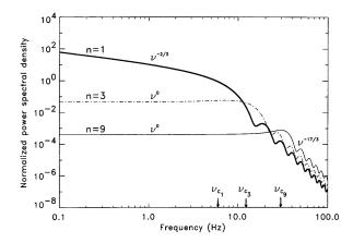
Figure 1.1: Zernike polynomial mean temporal power spectra in a given radial degree n for n = 1, 3, 9. The asymptotic power laws and the cutoff frequencies (here noted by  $\nu$  instead of f in the text) are indicated. Credit: Conan et al. (1995).
