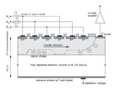
Figure 3.3: Schematic cross-section of the PNCCD. The full volume is depleted and the charges are collected in the potential minimum defined by the three  $\phi$  voltages, which after collection allow, by appropriate clocking, the charge transfer to a readout anode and a first on-chip amplifier. Credit: Hartmann et al. (2005).
