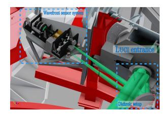
Figure 2.4: CAD layout of the dichroic setup in front of the LUCI rotator structure directing the laser beams to the WFS. The laser beams are represented in green. Courtesy: figure annotated from L. Busoni and M. Bonaglia.
