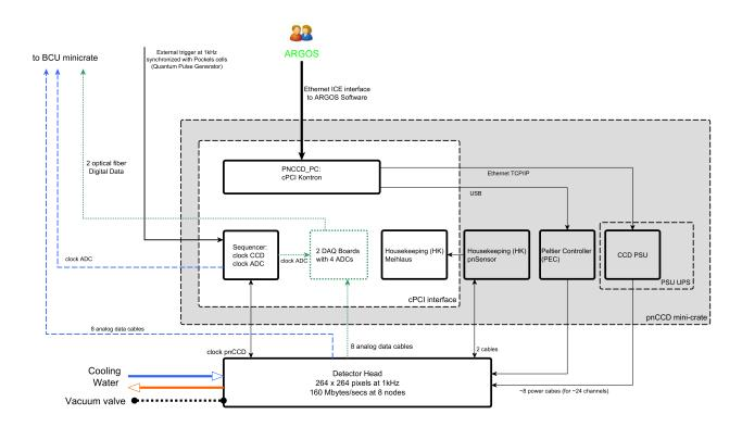
Figure 3.7: Interface scheme of the ARGOS PNCCD unit. It displays all interfaces between the PNCCD mini-crate and the PNCCD camera head. The two ADC possibilities are also represented : (dotted green) using the optical ADCs; (dashed blue) the BCU built-in ADCs. See text for more details.
