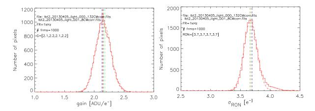
Figure 3.20: Gain and noise pixel histograms obtained from two (dark and light exposed) sets of 1000 frames with their fitted Gaussian distributions. The dark frames are full commonmode corrected by subtracting the average level over 132 pixels. The red curve is the distribution for the first CAMEX, the vertical lines indicate the mean values for each CAMEX unit. We can observe a "non-gaussianity" of the RON distribution at the high end. This is further discussed below.
