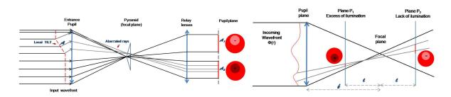
Figure 1.5: (Left) Pyramid WFS concept sketch (2D). A local phase tilt causes the aberrated rays to hit one side only of the pyramid causing pupil images non-uniformity between the four images. See text for more description. (Right) Principle of the curvature wavefront sensor. An local aberration (curvature) leads to a difference of illumination between the intra- and extra- focal plane P1 and P2. See text for more description. Credit : both sketches are from Aller Carpentier (2011).
