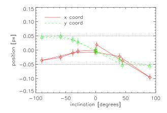
Figure 3.14: Result of a tip-tilt test with the final camera model. This is obtained from a centroid measurement on the chip. The total flexure tip-tilt amounts to  $\sim 0.1$  pixel= $4.8 \mu$ m and is therefore within our specifications. See text for more details.
