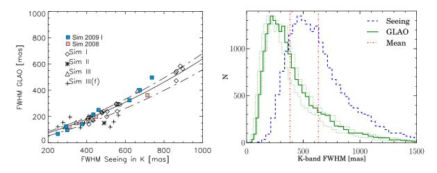
Figure 2.1: (Left) ARGOS performances evaluation based on closed-loop and ARGOS optics simulations. We can observe the factor of 2-3 improvement in the PSF FWHM. (Right) Predicted reduction of the PSF size in the K-band based on seeing statistics as derived at the MMT in Arizona. The mean of the distribution before and after GLAO (0.63'' and 0.34'' respectively), correction are indicated in red. Credit: ARGOS consortium (2009, 2010).
