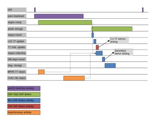
Figure 4.9: Conceptual data flow diagram of the ARGOS BCU from first pixel download to slope finalization and diagnostics savings. The latency is calculated from the final pixel download to the final slope construction. The synchronization is done through real time communication, *i.e.* the start-of-frame (SOF) is given by the start of a PNCCD frame. This representation is only indicative and we refer to the text for proper timing estimations. Credit : Andrighettoni & Biasi (2011).
