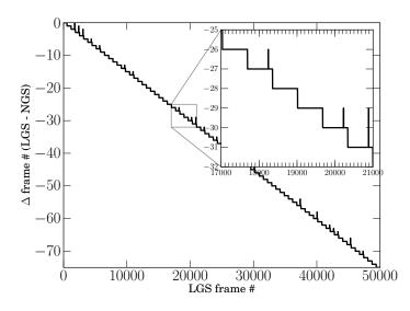
Figure 4.4: Difference of the frame numbers between the PNCCD frame (here simulated by the framegenerator) and the NGS tip-tilt frame for 50 seconds. Regular steps are  $\sim 660$  counts appart, and glitches of 1 to 2 counts can be seen. See text for discussion.
