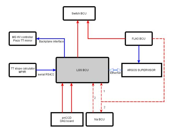
Figure 4.1: Sketch of the ARGOS WFS computer interfaces (LGS BCU). The red lines designate fast optical links. The dashed red lines represent two variants. The nominal possibility (1) featuring an interface with the FLAO BCU, *i.e.* the pyramid NGS WFS. The second possibility (2) is foreseen for the "upgrade path", featuring a Sodium laser guide star, in which case the FLAO is pipelined through the Na BCU. We refer to the text for further details on the interfaces.
