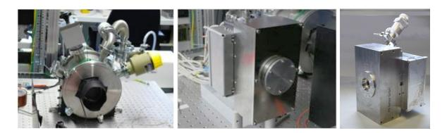
Figure 3.12: (Left) Initial camera housing inheritated from X-ray application. It required constant pumping and cryogenic cooling. (Middle) First "Engineering" housing model developed by PNSENSOR with a front side housing opening. (Right) Final housing model including its backside electronics and vacuum valve.
