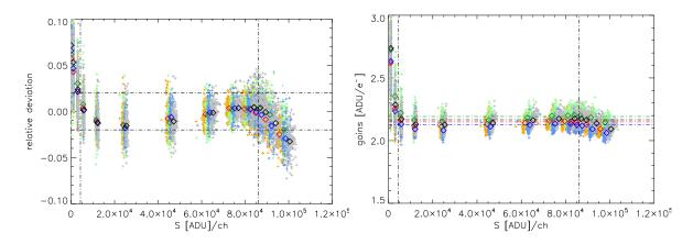
Figure 3.19: (Left) Relative deviation from linearity obtained by taking the difference between the data and the photon-transfer curve fit. The horizontal dashed-dotted lines indicate  $\pm 2\%$ . (Right) Gain non-linearity. The horizontal lines indicate the average gain values. The vertical lines indicate the photon-noise dominated regime from one  $\sigma_{eRON}$  to saturation.
