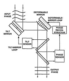
Figure 1.4: Essential components of an adaptive-optics system. The phase sensor measures the phase difference between the incoming wavefront and the surface of the deformable mirror. A separate tip-tilt sensor is used to correct for the image motion. Credit : Parenti & Sasiela (1994).
