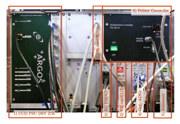
Figure 3.9: Final ARGOS PNCCD minicrate. This includes essentially 1) the CCD power supplies, 2) a cPCI computer hosting the software for remote operation, , 3) 2 housekeeping boards, 4) two ADCs with optical output, 5) a pattern generator (or sequencer), and 6) the Peltier controller for the camera cooling.
