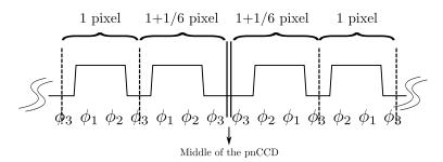
Figure 3.11:  $\phi$  registers in "collecting", or storage, mode along one channel in the middle of the PNCCD. The double middle lines define the middle of the PNCCD, where the left side is readout to the left, and vice-versa for the right. The dashed line defines the separation between pixels along the channel. This  $\phi$  configuration provides better pixel uniformity but leads to larger central pixels, by an additional factor of 1/6.
