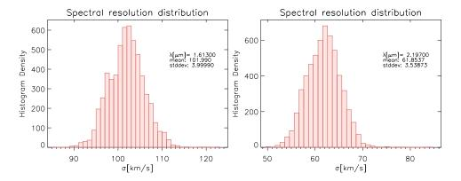
Figure D.2: Measured spectral resolution in the H and K-bands (by Gaussian fitting of unblended sky lines at 1.613 and 2.197 $\mu$ m) as measured on the initial data cube (no binning and masking). Dispersion in resolution is  $\sim 3.5$ -4 km/s.
