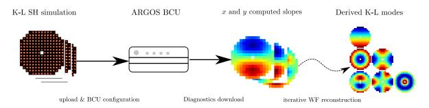
Figure 4.5: Sketch of the configurability and computation demonstration of the BCU. A set of appropriately simulated Karhunen-Loève (K-L) modes is first uploaded to the BCU, the BCU is then configured and the computation triggered. From the downloaded diagnostics, we retrieve the slopes and compute the wavefront by a simple iterative algorithm, as presented in the text. As expected we recover correctly the simulated modes.
