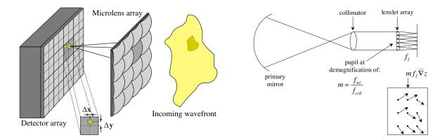
Figure 1.6: Shack-Hartmann concept sketchs. (Left) The incoming wavefront is subdivided by the microlens array, and image centroids are shifted according to average local wavefront slopes. Credit: Glindemann et al. (2000). (Right) The inset indicates typical displacement of the subimages proportional to the phase derivative. Credit: Chanan (2000).
