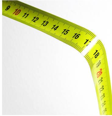
Figure 1.3: Folded configuration of a tape spring.
