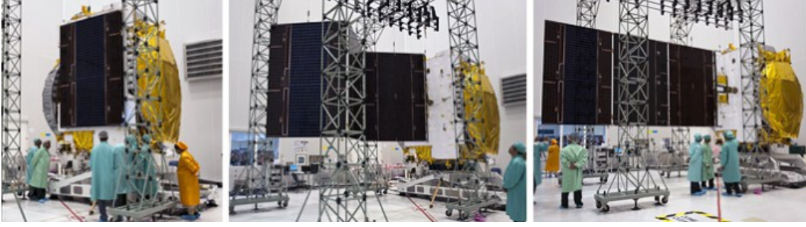
Figure 5.3: On-ground deployment of the solar panels on GSAT-10 with a gravity compensation system [1].
