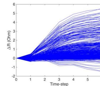
Cross-borehole ERT data are collected during the heat tracing experiment and change in electrical resistance are monitored. The simple linear relationship linking temperature and electrical conductivity is used to model geophysical data from groundwater transport simulations required by PFA.
