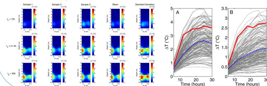
ERT data are used to forecast the spatial distribution of temperature in the aquifer. The correlation is high since data and forecast are colocated. The posterior distribution of temperature is validated using direct measurements in piezometers within the ERT panel.
