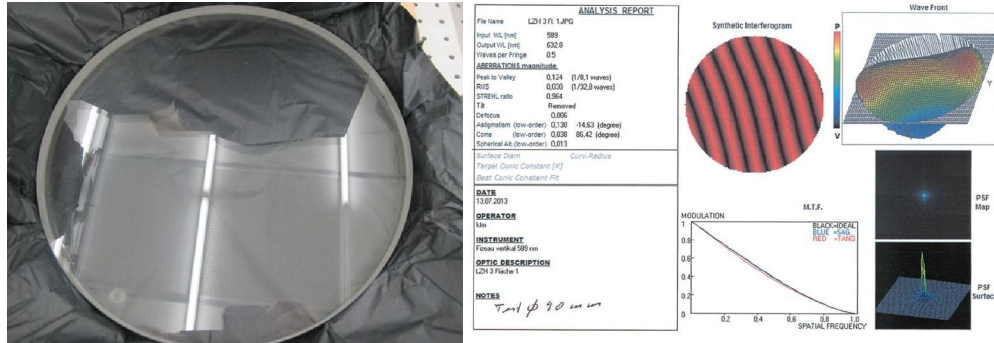
Fig. 2. Left: picture of one of the ARGOS dichroics before the coating process. Right: measure of the third dichroic surface error performed at LZH on a 90mm diameter patch. The surface PtV amounts to 1/8 waves, mainly due to an astigmatism term.
