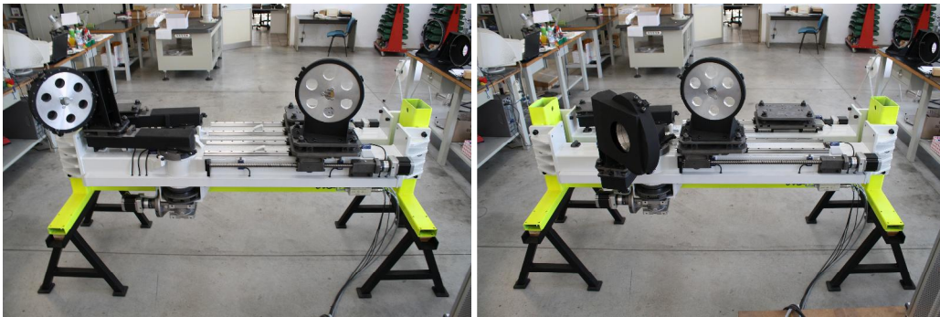
Fig. 4. Picture of the ARGOS laser pick-off support structure assembled at Tomelleri s.r.l. premises. The 2 cells are holding aluminium dummies of the optics to test the stability of the structure under different gravity conditions. Picture on left shows the parked position for the optics while on the right it shows their working positions.
