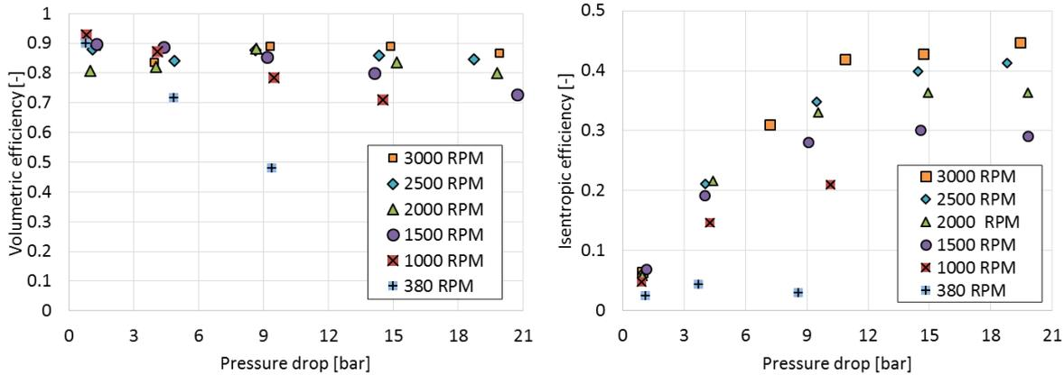
Fig. 3. Performance of the gear pump a) volumetric efficiency b) isentropic efficiency
