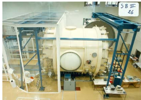
480 m 2 and 10 meters high clean room. Equipped with a bridge of 5 tons, it will house the new space simulator "FOCAL 5".
