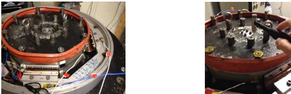
Figure 4: Hammer impact testing on the shaker in vertical configuration
