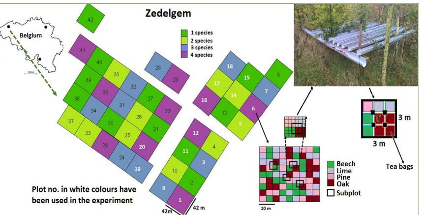
Fig. 1: Layout of the Zedelgem site of FORBIO plantations with detailed plantation design of a 4 species mixed plot. A 3 m × 3 m rainout shelter has been built around beech and oak trees to impose drought. Details about FORBIO see Verheyen et al. (2013).
