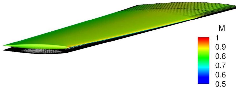
Figure 7: Static aeroelastic deformation of the AGARD 445.6 wing. The initial configuration is in gray. Contours of the Mach number are superposed to the deformed wing.
