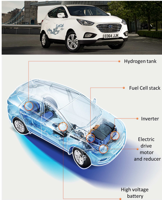
Figure I-4: (Up) A photography of the ix35 Fuel Cell (the first mass production model of Huyndai) and (Down) the key parts of the motion technology 4 .
