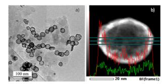
a) TEM micrograph of Pt-Co hollow particles/CX, and b) EDX line-scan of a single hollow particle, the profiles show Pt (red profile) and Co (green profile) over the entire particle. The obtained image corresponds to the projection of a hollow shell as indicated by the lack of signal in the center.
