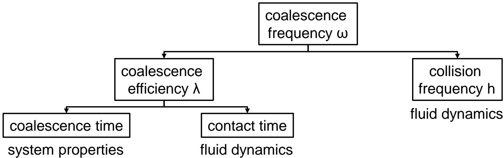
$$\omega = \lambda \ h = h \exp\left(-\frac{t_{coalescence}}{t_{contact}}\right)$$
