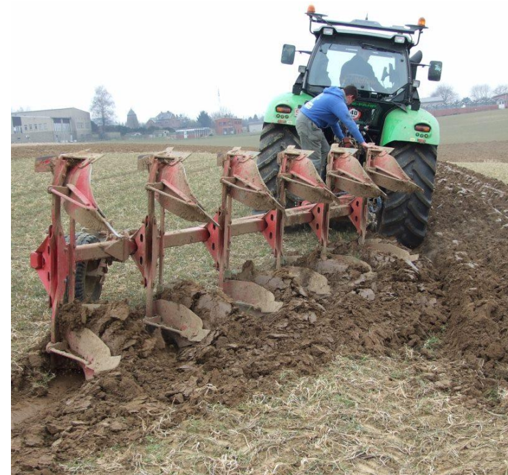
Figure 11 Moldboard plow employed on CT plots to mix and invert soil to a depth of 25 cm. Image credit: Marie-Pierre Hiel.
