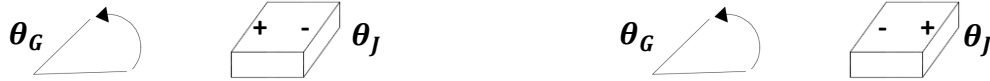
Figure B-13. The position of the inclinometers in rapport with the global system of coordinates
