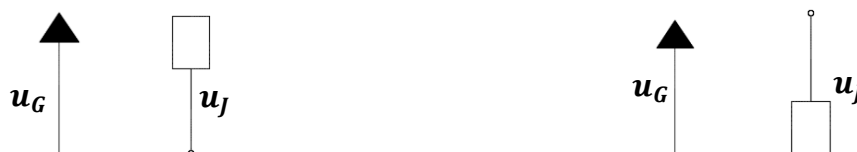
Figure B-10. The position of transducer compared with the axis of the GSC
