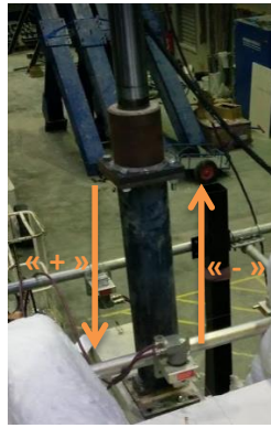
Figure B-5. The sign convention for jacks
