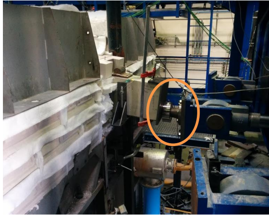
Figure 6-56. The load cell placed on the horizontal jack
